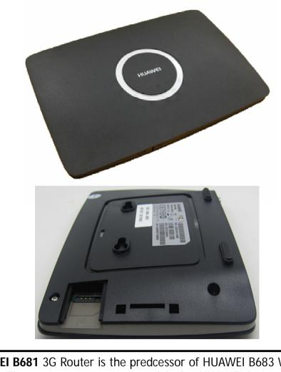
**HUAWEI B681** 3G Router is the predcessor of HUAWEI B683 Wireless Router. There are many variant models for HUAWEI B681, such as HUAWEI B681-44, HUAWEI B681-20, HUAWEI B681-24, HUAWEI B681-54 etc..The B681 Router could support download speed up to 21Mpbs and upload speed to 5.76Mbps. There are two RJ45 ports allowing two computers to connect simultaneously via Ethernet cable. And One RJ11 is for WLAN cable.
